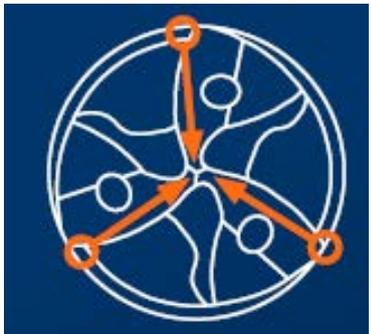
**Photo caption:** On the GARANT MasterSteel FEED solid carbide drill, the self-centring forces act on three cutters instead of just two.
