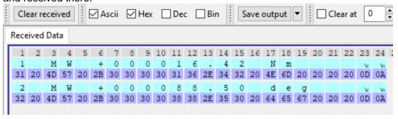
The first line with green background shows the torque measured value with the unit "Nm", the second line with green background shows the angle measured value with the unit "deg". The two lines with a purple background represent the characters as hexadecimal values (according to ASCII).
