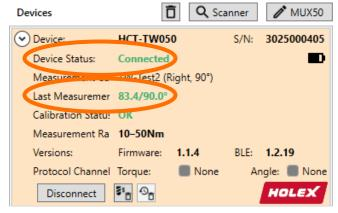
The HCT Windows App and the Bluetooth wireless technology used allow you to connect a maximum of 16 HCT tools. Please note, however, that the connection setup and data transfer is delayed with so many HCT tools. We therefore recommend that you do not connect more than 10 HCT tools to the HCT Windows App. If you use more HCT tools, distribute them to several workstations and thus to several PCs with the HCT Windows App and HCT dongles.
