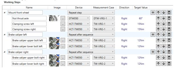
Finally, save the working plan to the database by clicking "Save" in the top line of the HCT Windows App.
