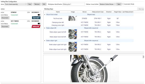
The measuring cases are now transferred step by step to the HCT tools according to the working plan and the HCT Windows App waits for the execution of the measurement case and its confirmation with the send button. Then the HCT Windows App jumps to the next measurement case etc.
